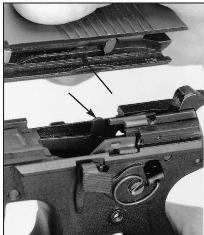
A tab on the trigger lever engages a recess in the underside of the slide (arrows) to disconnect it from the firing lever during slide cycling. Trigger must be released for trigger lever to re-engage. Note firing pin block plunger in the underside of the slide.
