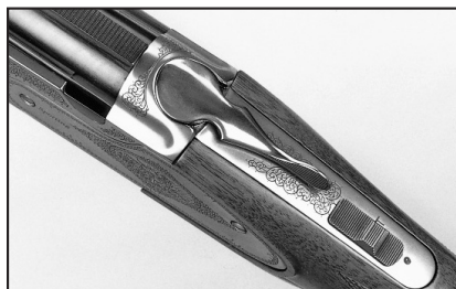
The tang-mounted barrel selector is behind the top-lever. The gun's triggers, both a crisp 5 lbs., were a pleasant surprise.
