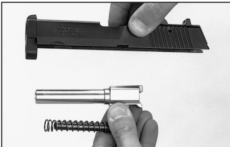
Disassembly of the Golan continues with the release of the slide by depressing the decocking lever and pulling it, along with the barrel and recoil springs, forward off the frame. The barrel, recoil spring and its guide can then be removed from the slide.
