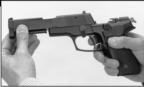
Disassembly of the Golan continues with the release of the slide by depressing the decocking lever and pulling it, along with the barrel and recoil springs, forward off the frame. The barrel, recoil spring and its guide can then be removed from the slide.
